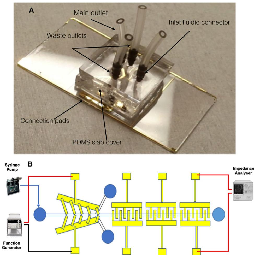
**Figure 2.** (A) Fabricated impedance biosensor devices sealed with PDMS slabs, (B) Schematic of the pathogen testing setup which consists of the syringe pump, the function generator, and the impedance analyzer.
