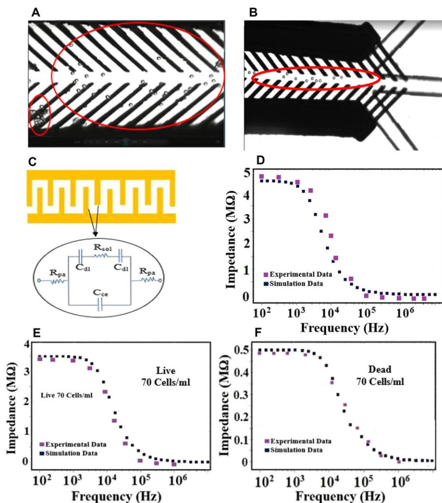
**Figure 3.** (A) Optical image of the microbeads moving in the focusing region before applying p-DEP forces, (B) after applying p-DEP forces, (C) Equivalent circuit of the impedance-based biosensor showing the circuit components, (D) The simulation of the equivalent circuit and the experimental results showing a good match of the experimental results with the simulated results for live *Salmonella* of 120 cells/mL, (e) live *Salmonella* of 70 cells/mL and, (f) dead *Salmonella* of 70 cells/mL.
