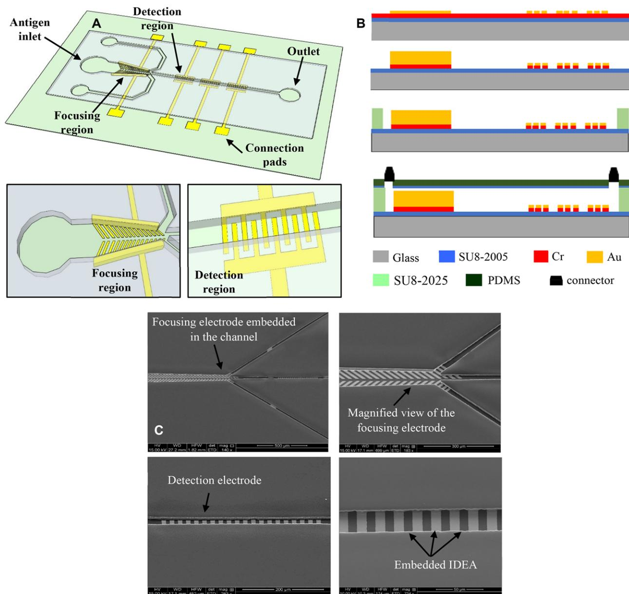
**Figure 1.** (A) Three dimensional schematics of the biosensor device showing the focusing and the detection regions, (B) Cross-sectional views of the biosensor fabrication processes, (C) SEM micrographs of the fabricated device showing the focusing electrodes, the detection electrodes, and the split of the microchannel.
